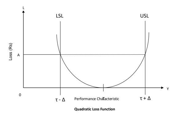
The quadratic function is shown in figure. In this situation, the loss occurs as soon as the performance characteristic, y, departs from the target  $\tau$ .
